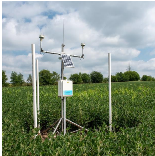
An IFC Hydrostation Measuring Rainfall and Soil Moisture
